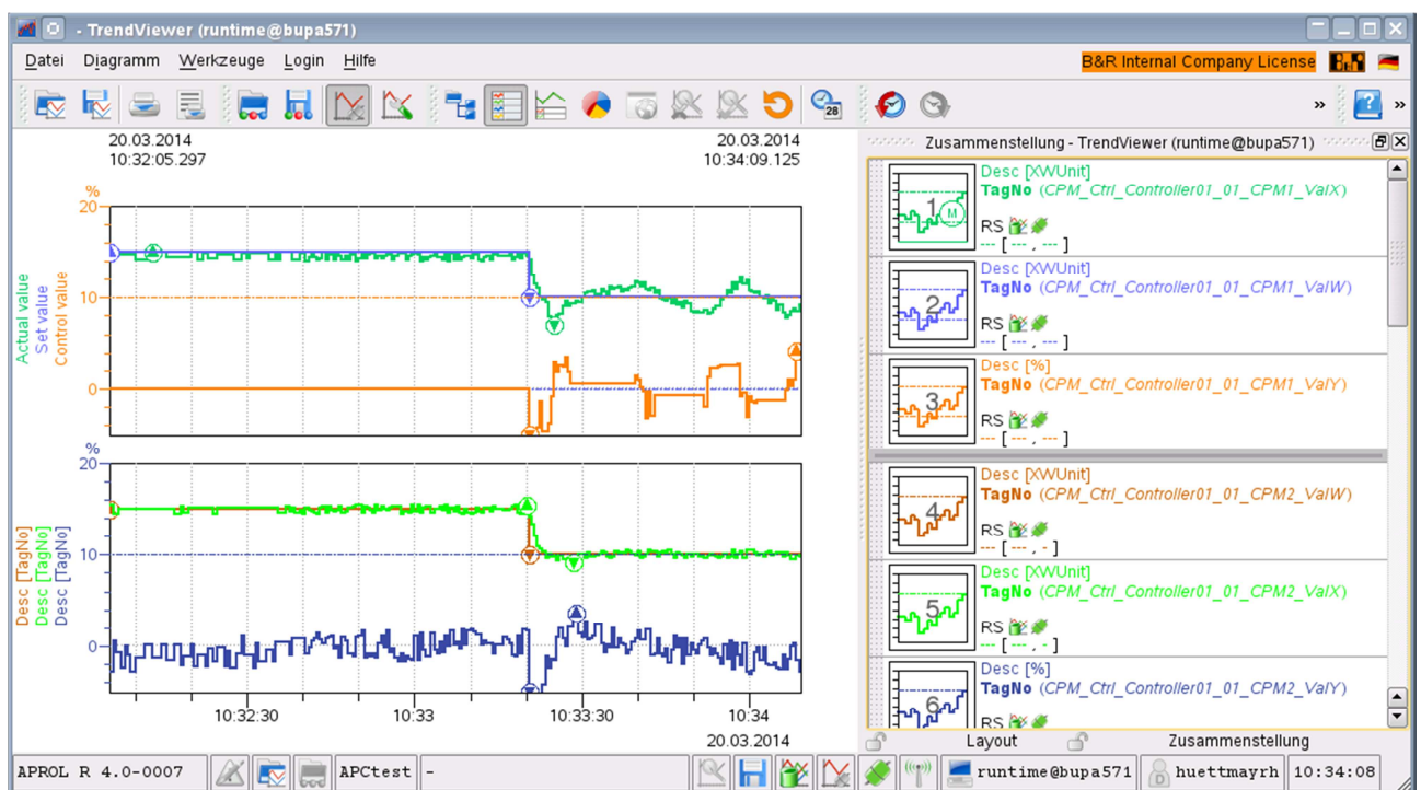
Figure 18, PID control with and without deadband (system without inherent regulation)
